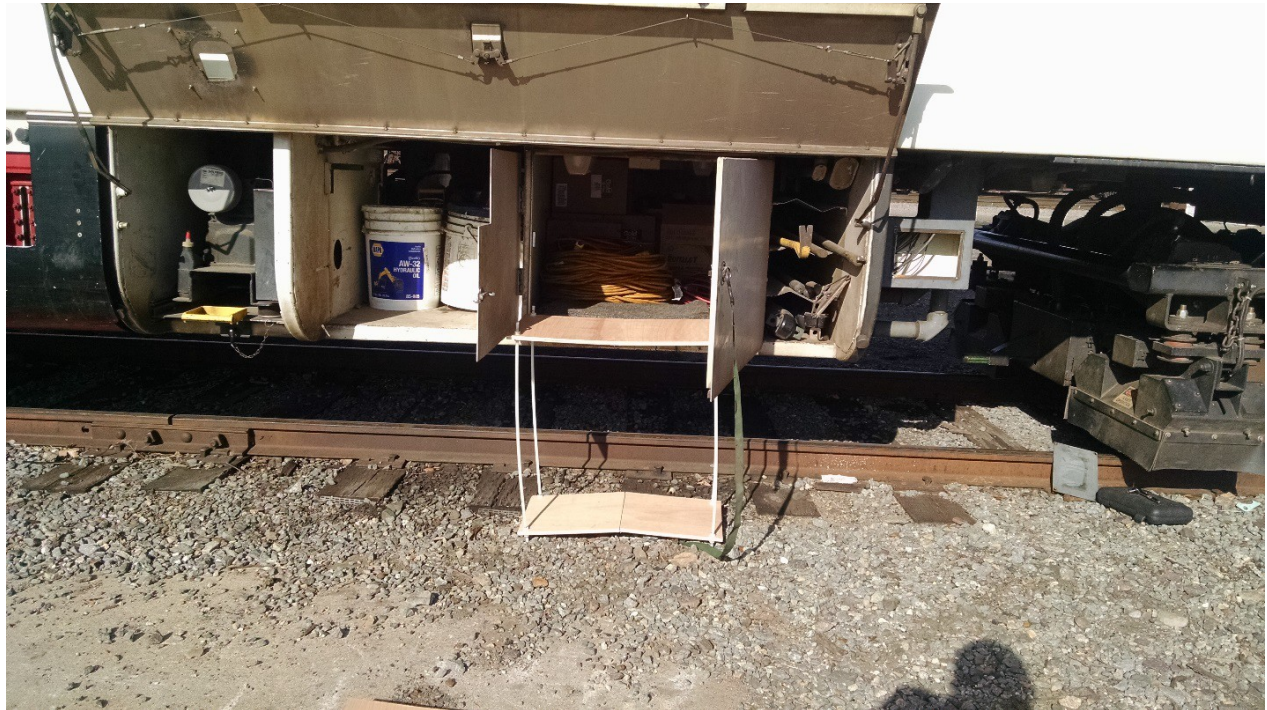
Figure A 1. DOTX220 storage compartment with plywood mockup of 2 GHz antenna
