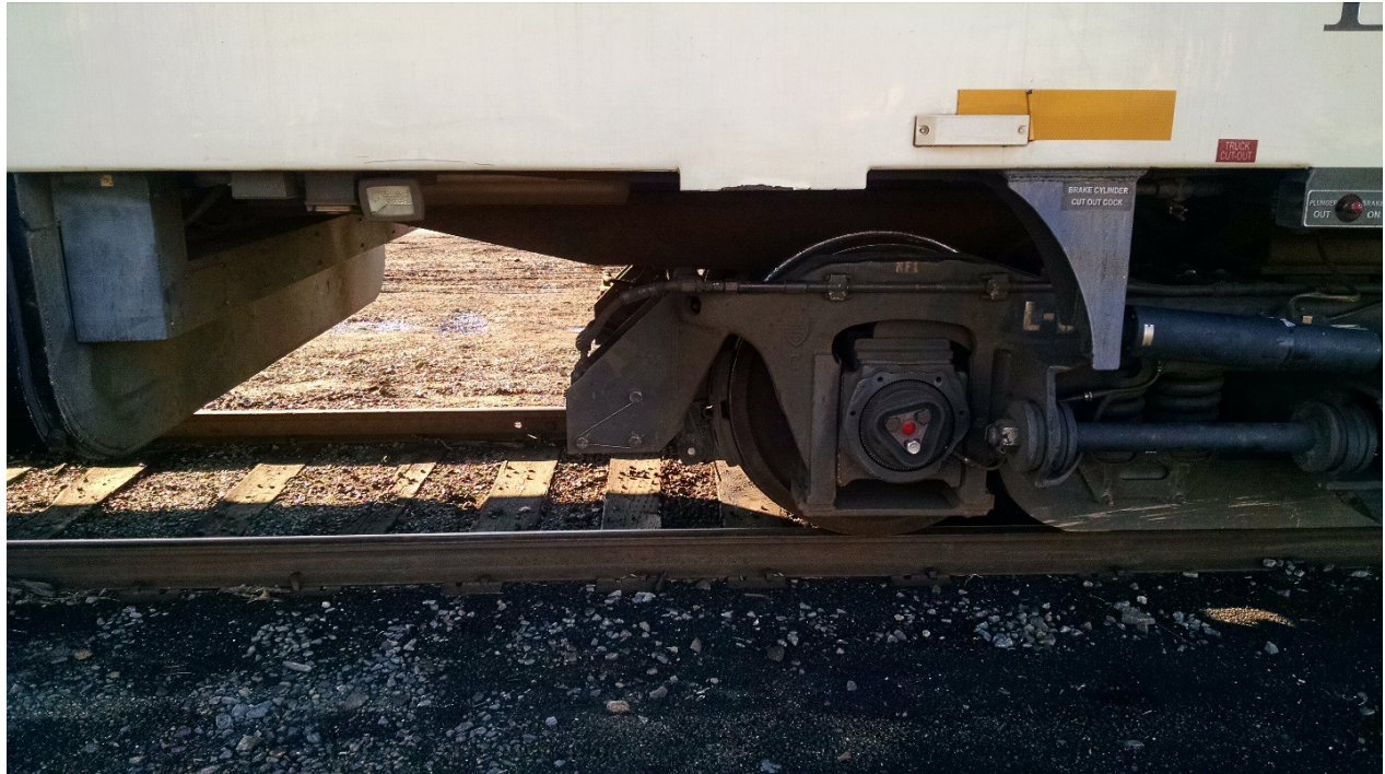
Figure A 2. DOTX220 available space between tank and rear truck
