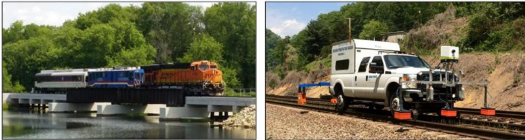
Figure E 1. (Left) FRA's track inspection cars, T218 and T220 in consist with BNSF locomotive. (Right) BBRI hi-rail inspection car fitted with six-channel GPR and mobile terrestrial laser scanner
