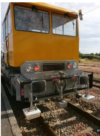
Figure 2 Georadar vehicle (Source: Ground Control Geophysik & Consulting GmbH)
