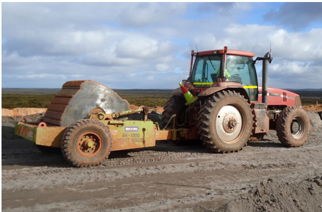
Figure 1. 8 t four-sided impact roller
