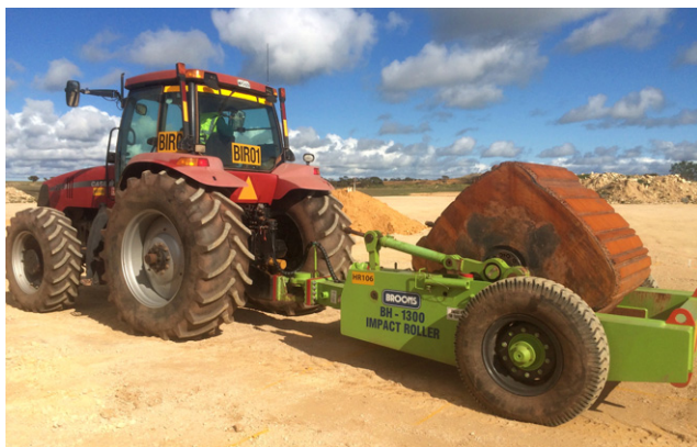
Fig. 1. Eight tonne four-sided impact roller
