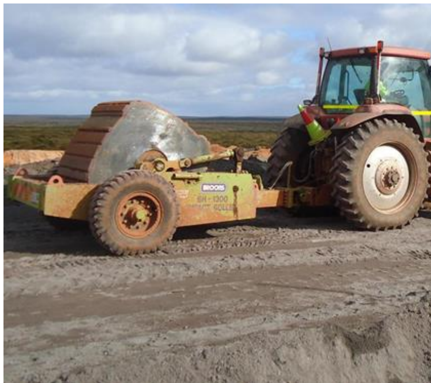
Figure 1: 8-tonne square impact roller
