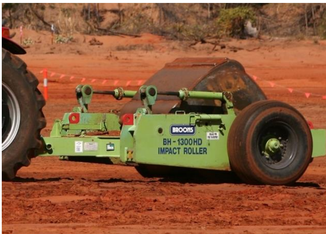
Figure 1. 4-sided impact rolling module
