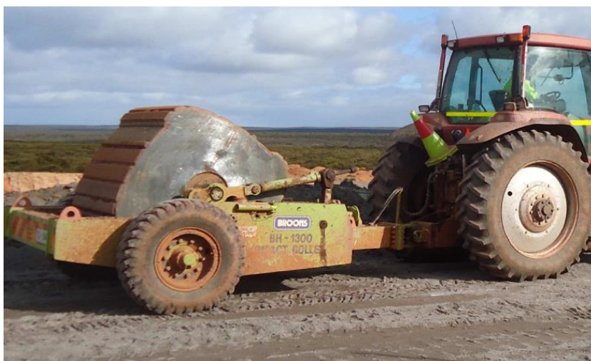
Figure 2. 4-sided RDC module (Broons).
