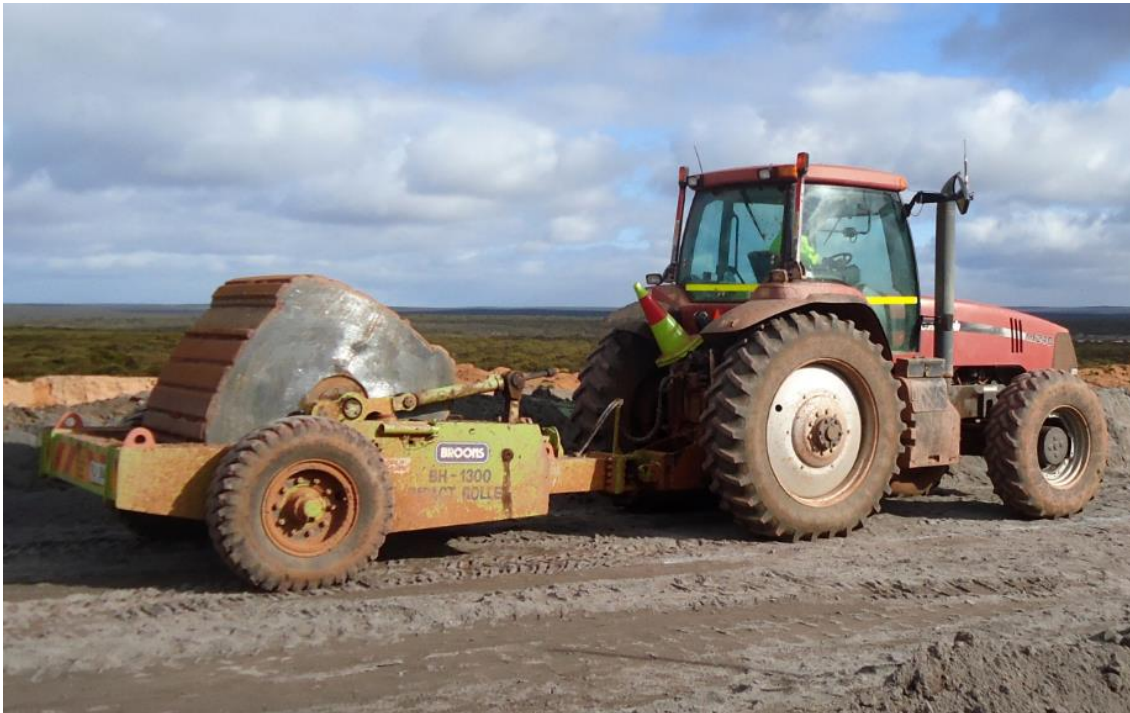
Figure 3.1: 8-tonne 4-sided impact roller
