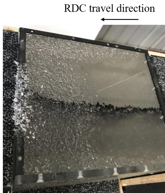
Figure 2.15: Particle surface after 40 passes of the 3.64 kg module travelling at 256 mm/s.
