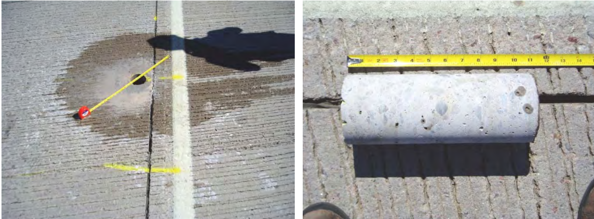
Figure 19. Diagonal orientation of tie bar across joint (left) and the 11-in. core (right).
