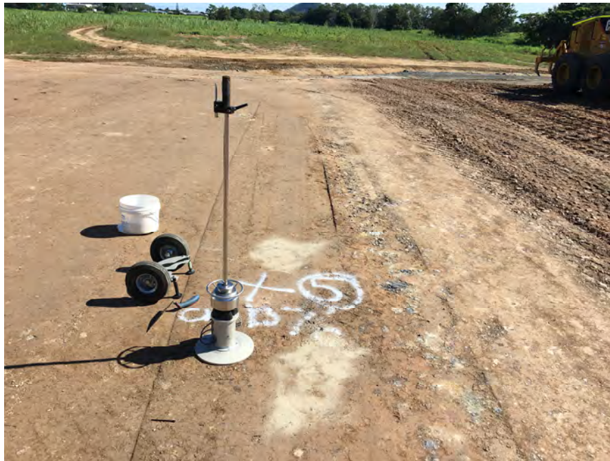
Figure 10-1 A density pass with a fail LFWD disagreement area
