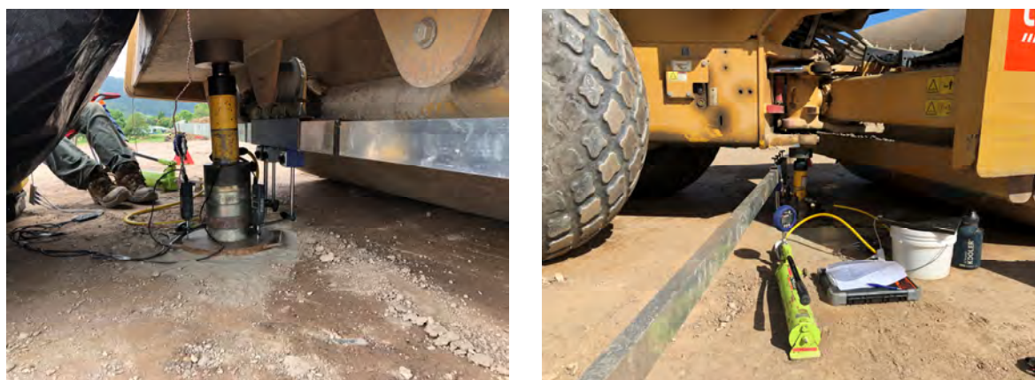
Figure 7-1 Pictures of the equipment arrangement typically adopted onsite for PLTs setup (note the presence of the independent reference beam for measurement of observed settlements and jacking against external reaction force)
