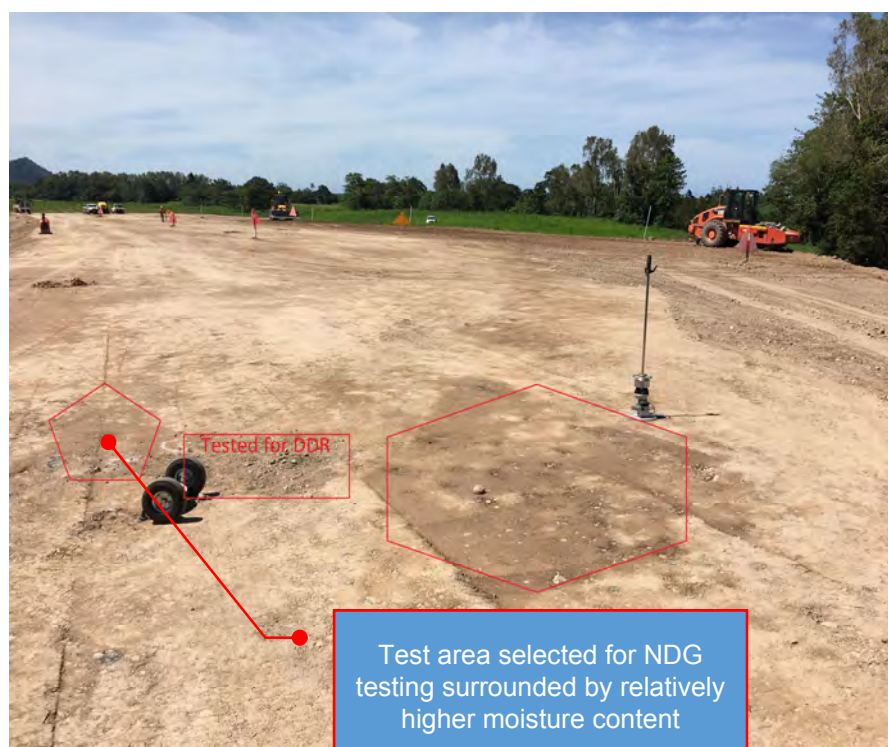
Figure 10-2 A density pass does not "notice" adjacent wet spots
